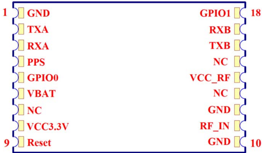
Figure 2: SM1110-MTBD Pin Package
